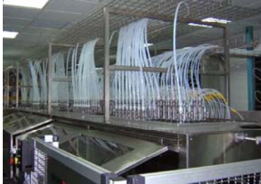
Blending systems for the automated mixing of aromas, scent extracts or chemicals; separate tanks and lines are necessary for each base material.
